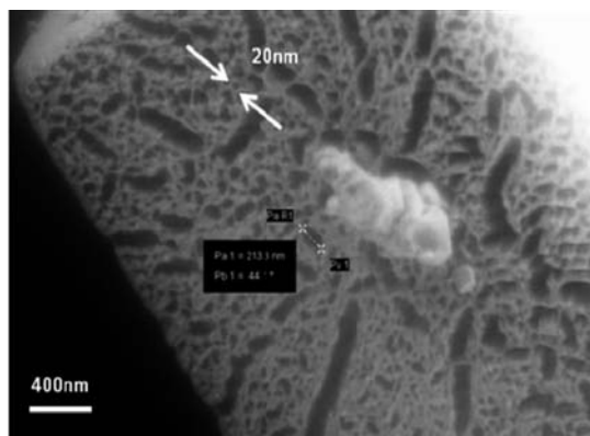
Figure 10. SEM image of Ni(bdc)(ted) 0.5 showing macro- and mesopores ranging from ~20 to 200 nm. The small pores of 20 nm are believed to cause the shift on the Q dip in gaseous H 2 . This is caused by the perturbation of the gas phase by the MOF walls affecting the IR activity of the gas phase induced by intercollision interference.
